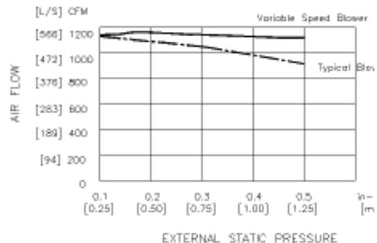
**The AEPT air handler delivers the optimum air flow for the system size, whether in heating or cooling mode, regardless of the static pressure imposed by the air distribution.**
